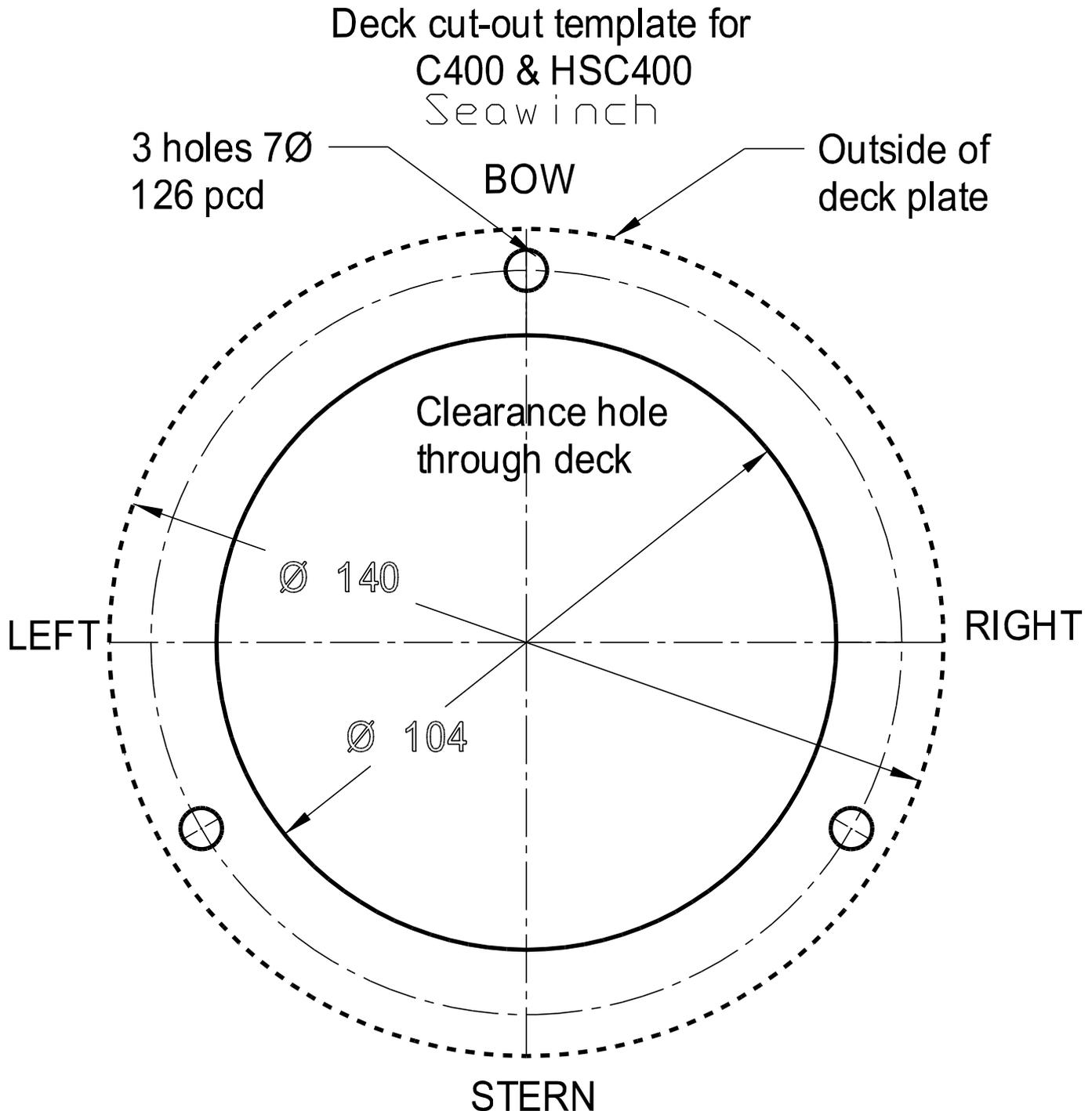
Standard studs will suit decks up to 30mm thick
